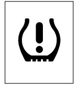
As an added safety feature, your vehicle has been equipped with a tire pressure monitoring system (TPMS) that illuminates a low tire pressure telltale when one or more of your tires is significantly under-inflated.
